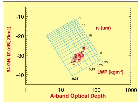
olution of 500 meters between the surface and 20 km altitude with an effective radar footprint of 1.4 km (cross-track) x 4 km (along-track). An alternate, pulse-compressed mode allows a vertical resolution of 250 m between 5 and 20 km altitude. The nominal detectable reflectivity factor is approximately -29 dBZ.
