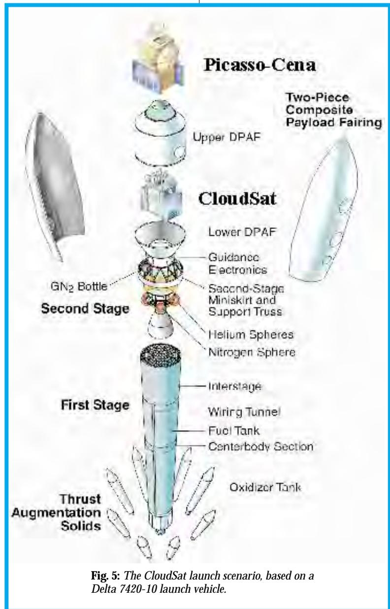
**Fig. 5:** The CloudSat launch scenario, based on a Delta 7420-10 launch vehicle.
