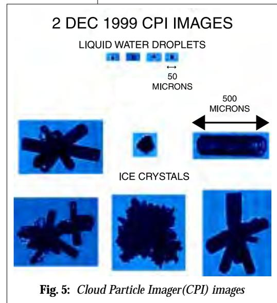
**Fig. 5:** Cloud Particle Imager (CPI) images
