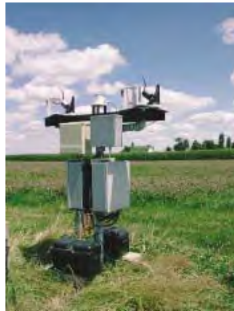
Figure 1b: The shadow-band radiometers use a computer-controlled, automatic rotating shadow-band, which determines near-simultaneous measurement of total horizontal, direct normal, and diffuse radiation at each filtered passband. The broadband UV meters measure ultraviolet radiation in the UV-B spectral range of 280-330 nanometers.
