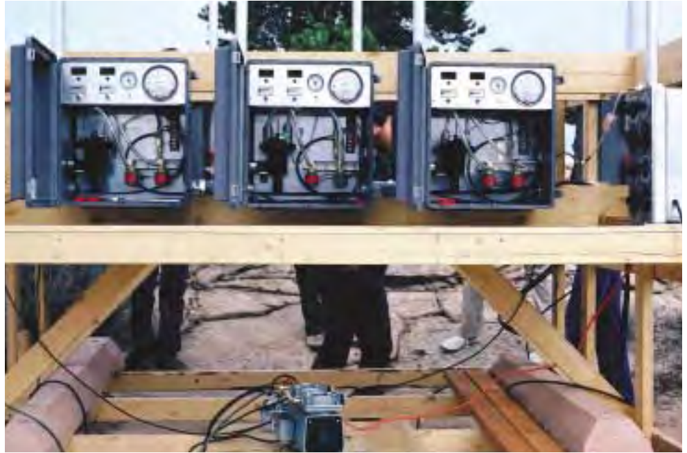
Close-up of a typical IMPROVE aerosol sampler. Each of the three different modules collect fine particulates on different media and are subjected to various chemical analyses to characterize the amount of chemical species in the air.
