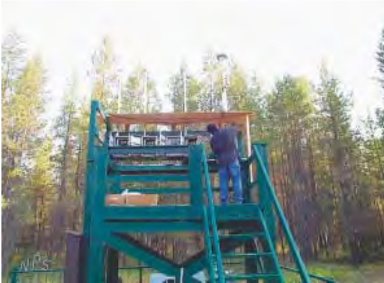
Photo of the IMPROVE site in Glacier National Park. Visible are the three different modules collecting aerosol for chemical speciation.
