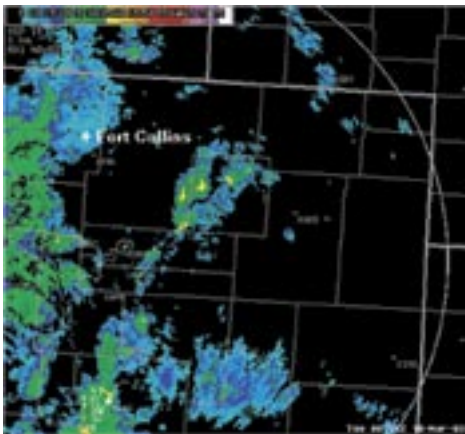
Figure 4. One line of convection moves off to the west of Fort Collins (squall lines were moving westward) as a second line forms to the east. Figure shows the 0.5 degree tilt, PPI reflectivity scan taken from the Denver, Colorado WSR-88D at around 6:00 pm on the evening of 17 March 2003.
