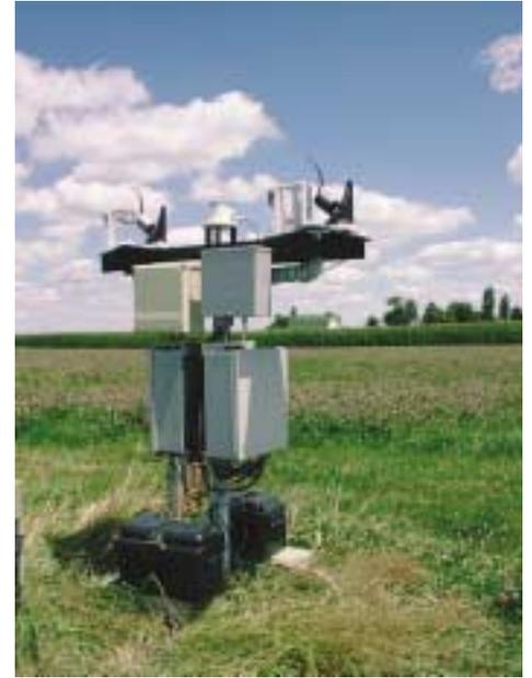
Figure 1b: The shadow-band radiometers use a computer-controlled, automatic rotating shadow-band, which determines near-simultaneous measurement of total horizontal, direct normal, and diffuse radiation at each filtered passband. The broadband UV meters measure ultraviolet radiation in the UV-B spectral range of 280-330 nanometers.
