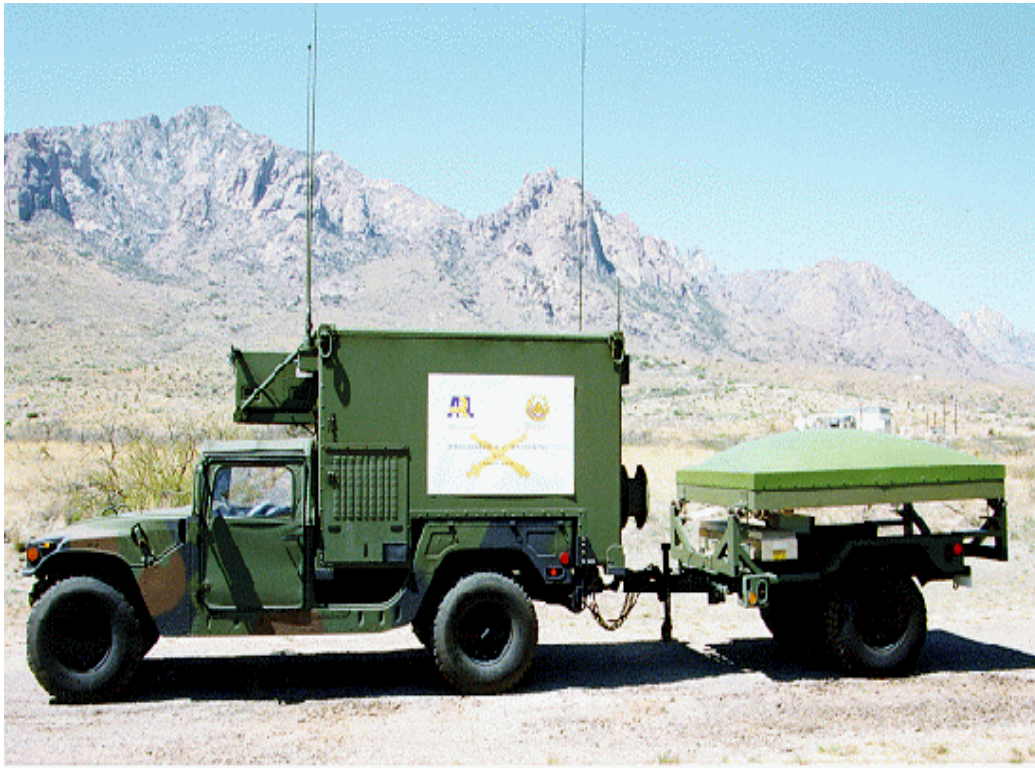
Figure 2. Photograph of the 924 MHz wind profiling radar antenna towed by HMMWV. Processing hardware and software are housed inside the HMMWV's shelter.
