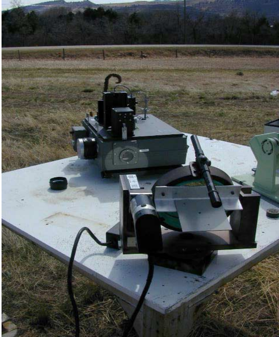
Photograph 1. Interferometer used to collect solar transmittances using various fields of view.
